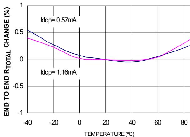
FIGURE 9. END TO END  $R_{TOTAL}$  % CHANGE vs TEMPERATURE
