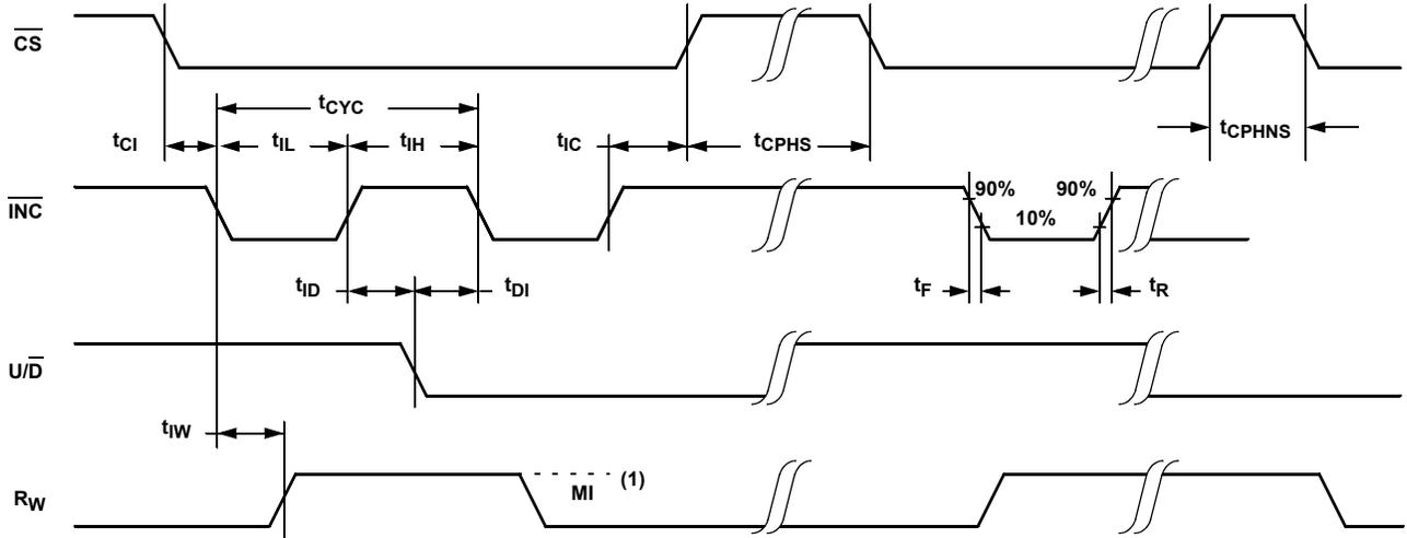
NOTE (1): MI IN THE TIMING DIAGRAM REFERS TO THE MINIMUM INCREMENTAL CHANGE IN THE WIPER POSITION.
