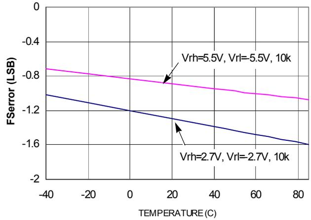
FIGURE 6. FSensor vs TEMPERATURE
