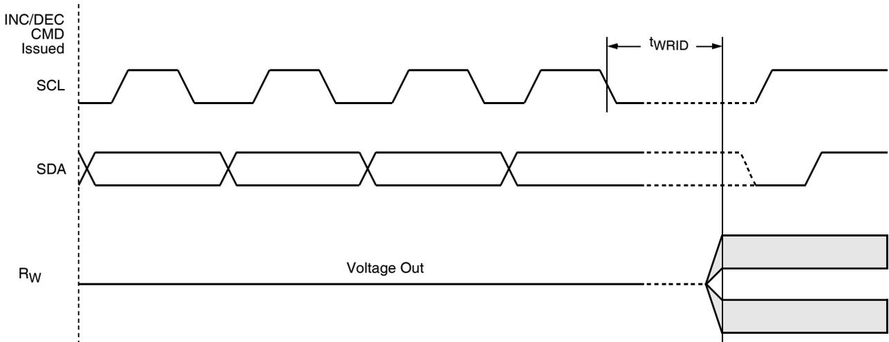
FIGURE 7. INCREMENT/DECREMENT TIMING SPEC
