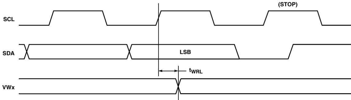
**Write Protect and Device Address Pins Timing**
