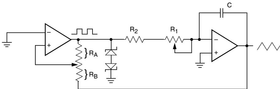
frequency  $\propto R_1, R_2, C$
