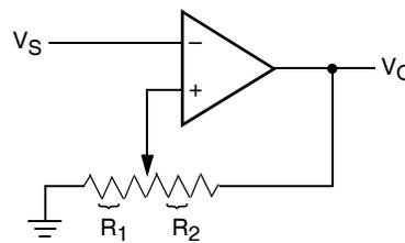
$$V_{UL} = \{R_1/(R_1+R_2)\} V_O(max)$$
