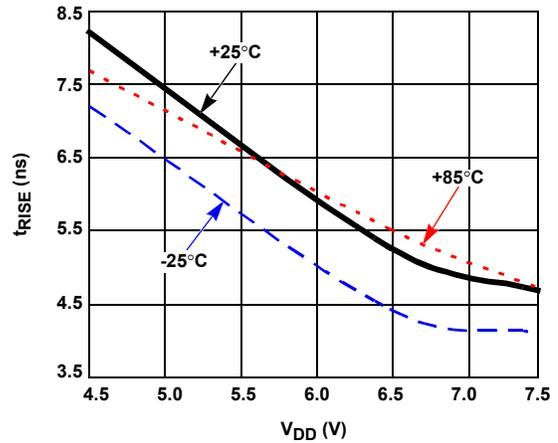
FIGURE 23.  $t_{RH}$  WITH TEMPERATURE ( $C_{GH} = 3nF$ , HSEL = BST)
