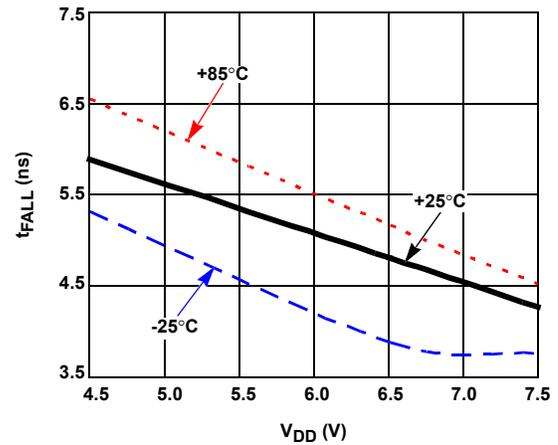
FIGURE 25.  $t_{FH}$  WITH TEMPERATURE ( $C_{GH} = 3nF$ , HSEL = BST)
