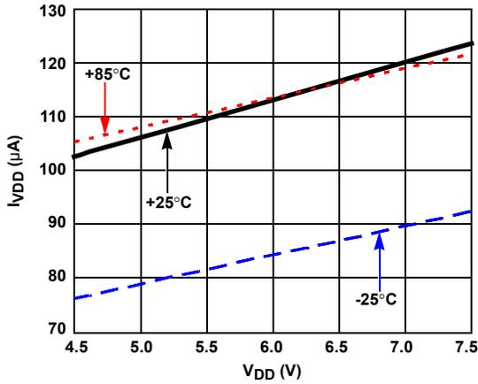
FIGURE 4.  $I_{VDD}$  vs  $V_{DD}$  WITH TEMPERATURE (NO SWITCHING)
