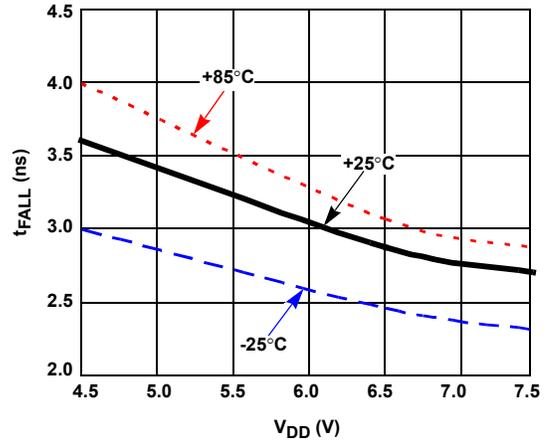
FIGURE 17.  $t_{FL}$  WITH TEMPERATURE ( $C_{GL} = 3nF$ , LSEL = VDD)
