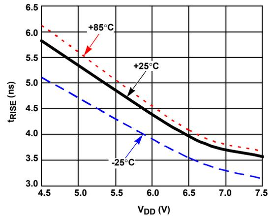
FIGURE 15.  $t_{RL}$  WITH TEMPERATURE ( $C_{GL} = 3nF$ , LSEL = VDD)
