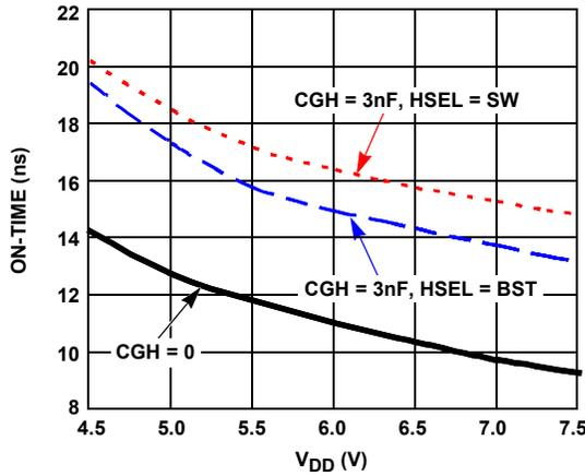
FIGURE 6. MINIMUM GH ON-TIME,  $t_{GH,ON}$  ( $T_A = +25^\circ\text{C}$ )
