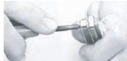
2. Apply a firm, steady pressure until the contact is released from the internal shoulder in the insulator. The shoulder of the tool tip bottom against the insulator face to prevent damage to the internal shoulder. Remove the tool tip and pull the contact from the rear of the connector. Repeat for the balance of contacts to be removed.
