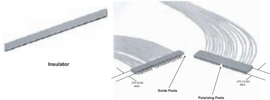
The guide posts and polarizing posts are inserted in the same manner as the contacts. The guide posts are inserted into the socket insulator and the polarizing posts are inserted into the pin insulator. The corresponding contact in the mating insulator must be removed for each. See assembly instructions.
