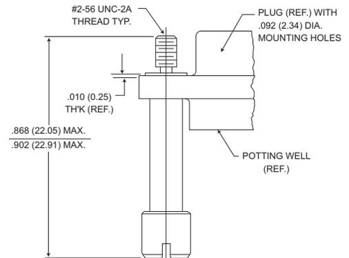
**Figure 2. Jackscrew - High Profile Slotted Head Size 9-51 Size 100\***
