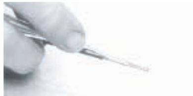
1. Place the proper insertion tip in the insertion/-extraction handle and put the tip over the wire as shown. The tool tip will butt up against the crimp pot. Connector must be firmly supported during both insertion and extraction operations.
