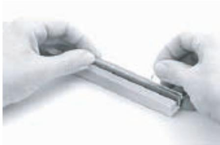
1. Place the connector into the slot in the assembly block with the arrows on the insulator pointing downward. The connector will bottom against the internal shoulder in the groove in the assembly block. Start contact insertion by placing the crimped contact in the cavity by hand.
