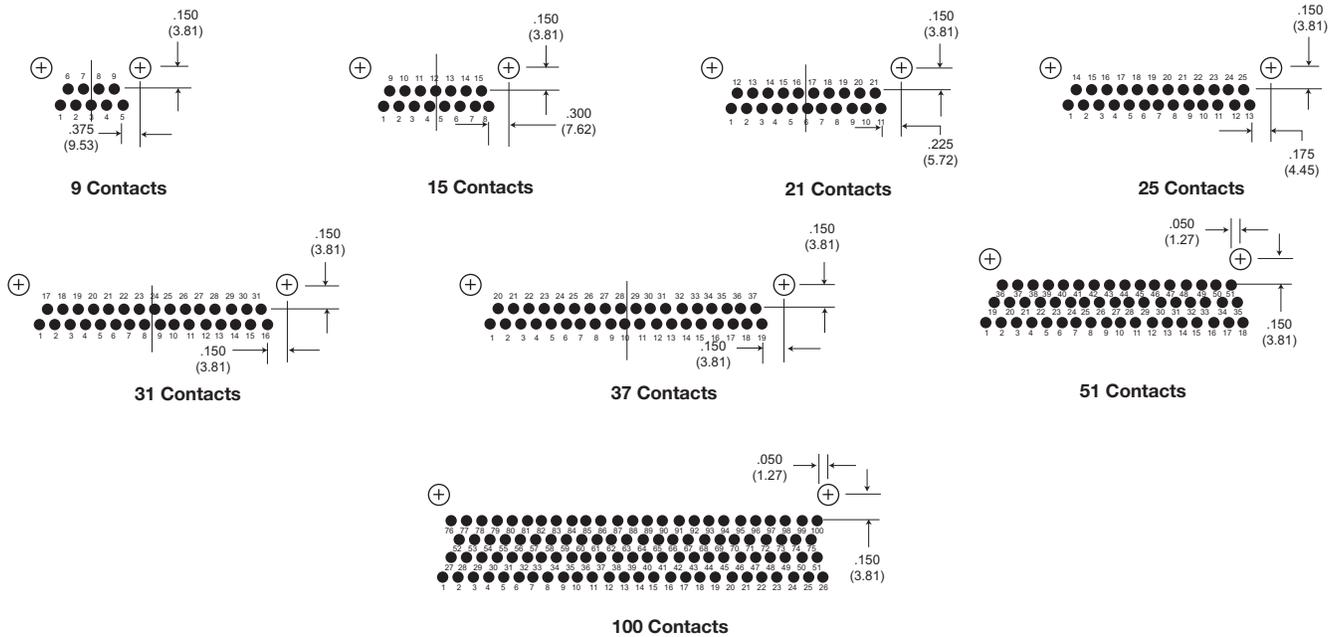
NOTE: Standard lead termination is #24 AWG, gold plated, solid copper, solder or tin dripped.
