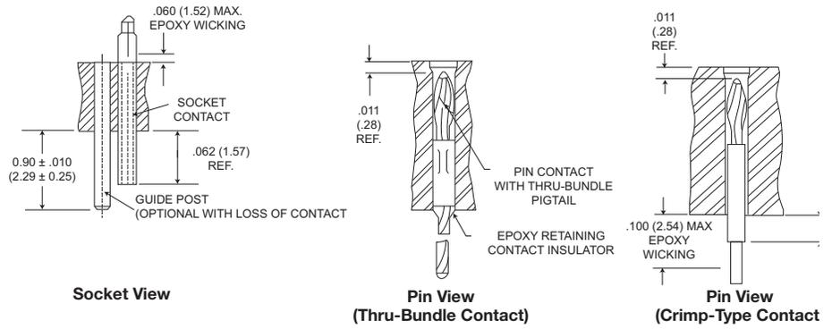
NOTE: Guide posts can be installed in any contact cavity for polarization purposes.
