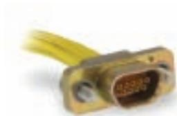
MDM connectors are used in applications requiring highly reliable, extremely small, lightweight connectors with higher density contact configurations than available in traditional rectangular connectors. They are available in 8 shell sizes accommodating from 9 to 100 contacts, and special arrangements of power and coaxial contacts.
