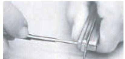
2. Using a firm, steady pressure, push the contact into the cavity until the resilient internal shoulder in the insulator snaps into the locking groove in the contact. The shoulder of the tool tip bottoms against the rear of the insulator, preventing over-insertion. Repeat for balance of contacts.
