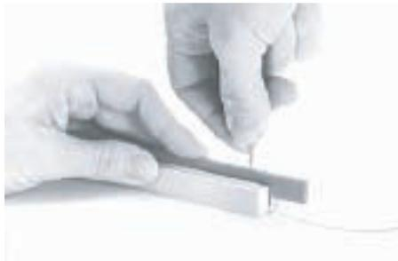
3. Insert the extraction tool into the cavity and apply firm pressure until the contact is pushed thru the rear of the connector.
