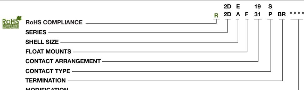
NOTE: Connectors may be ordered less contacts by adding the mod callout "FO" at end of number. Contacts are then supplied in bulk form.
