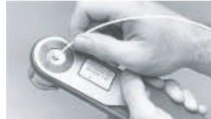
Using the proper crimp tool and locator, insert the contact into the locator. Insert the stripped end of the wire into the contact crimp pot, and crimp the contact to the wire. Squeeze the handles firmly to insure a proper crimp (tool will not release if crimping is incomplete).
