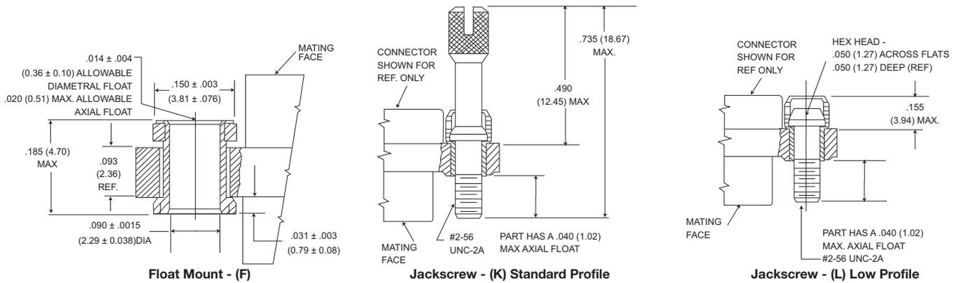
Shown here is a cutaway view of the float mount for the MDM connector. The basic shell dimensions are the same for the float mount and the screw mounting hole configurations. View shown is for standard float mount front panel mounting. Reverse mounting is available on request.
