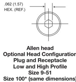
**Allen head Optional Head Configuration Plug and Receptacle Low and High Profile Size 9-51 Size 100\* (same dimensions)**
