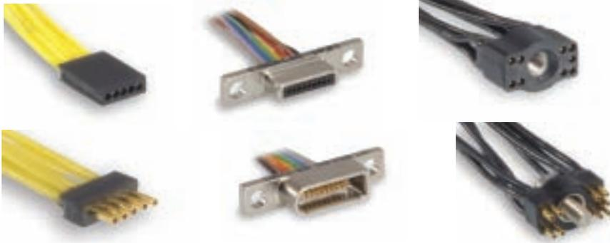
NANO contacts incorporate the highly reliable Twist Pin concept, which allows continuity in very dense areas and under severe shock and vibration, requiring low engagement and separation forces. Termination can consist of uninsulated pigtailed or insulated wire all pre-harnessed at our factory to your specifications.
