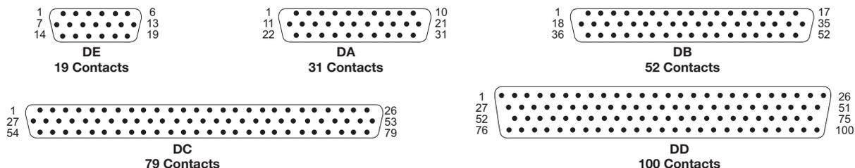
Cavity identification numbers are shown for reference only and do not appear on insulator front face. However they do appear on rear of insulator.
