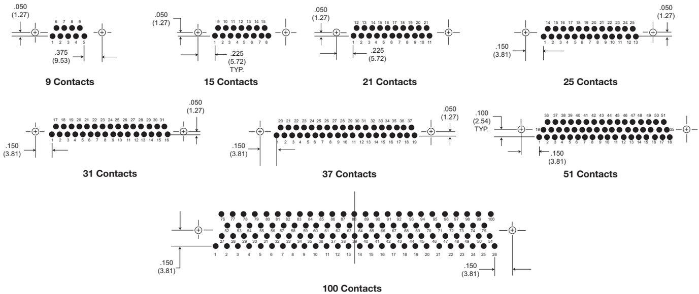
NOTE: Standard lead termination is #24 AWG, solid copper, solder or tin dipped
