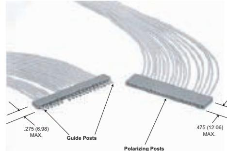
4. The guide post and polarizing posts are inserted in the same manner as the contacts. The guide posts are inserted into the socket insulator, and the polarizing posts are inserted into the pin insulator. The corresponding contact in the mating insulator must be removed for each.
