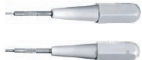
2. The pin extraction tool tip is tubular, slides over the pin bundle and butts against the front shoulder of the pin. The socket extraction tool is a solid rod that fits into the socket contact, the external shoulder butts against the contact socket shoulder.
