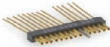
Modification code "-01" in the part number refers to guide posts located on both ends of the socket side of the 50-MIL STRIP connector and empty cavities on the pin side to accept the guide posts.
