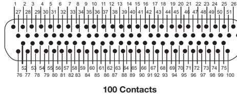
Contact identification numbers are for reference only and do not appear on insulator or connector body.
