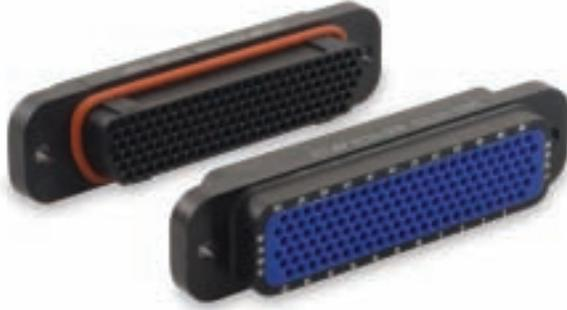
A subminiature all plastic high density "D" rectangular connector. The CDL is a general purpose connector with a peripheral o-ring and wire sealing gasket. Connector utilizes rear insertion, front release, crimp snap-in size 22, centi-loc contacts installable by the customer or, if preferred, by the factory.
