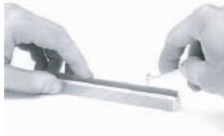
3. With firm steady pressure, push the contact into the cavity until the resilient internal shoulder snaps into the locking groove in the contact. To prevent over insertion, the tool tip bottoms against the rear of the insulator.
