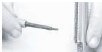
1. For contact extraction, remove the insertion tool tip and replace it with the proper extraction tool tip. (The socket tip will fit into the socket, and the pin tip will slide over the pin bundle). Insert the tool tip into the contact cavity: (the pin tip will butt up against the shoulder of the pin contact, and the socket tip will bottom out in the socket contact.)
