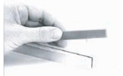
4. Lift the insulator from the groove and pull the contact out. Repeat for balance of contacts to be removed.
