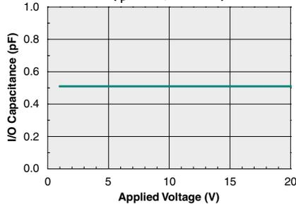
**Switch Capacitance vs. Applied Voltage**
