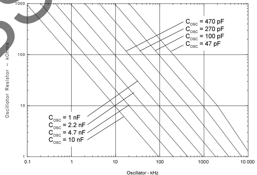
Fig. 4. Oscillator frequency component selection for IXDP630.
