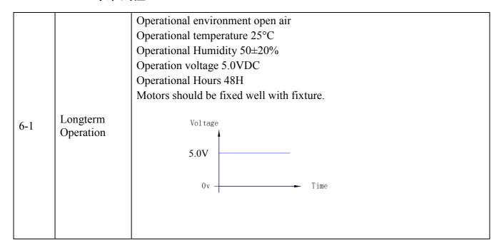
Before/After life test, measuring the rated load specification. Motor life is judged to come to an end. When
