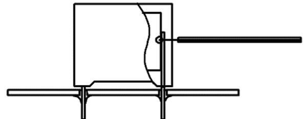
Temperature monitored inside the capacitor.
