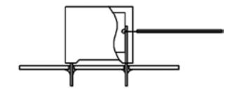
Temperature monitored inside the capacitor.
