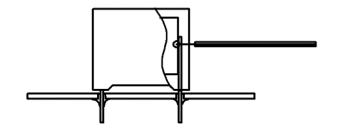
Temperature monitored inside the capacitor.
