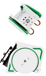
**STEP 2:** Clip the Servo:Lite board under the hooks on the inner side plates and slide it between the outer plates.
