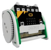
**STEP 4:** Secure the Servo:Lite board and micro:bit with the :MOVE T-piece.
