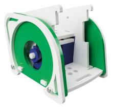
**STEP 8:** Add a wheel (built earlier) and screw the smallest servo screw through the middle to secure it.
