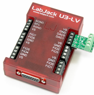
Figure 2: LJTick-OutBuff with U3-LV
