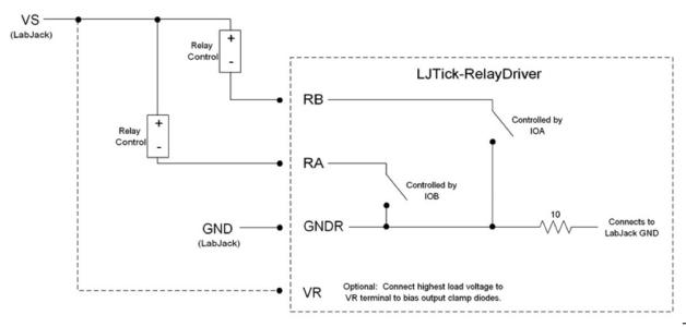
Figure 6: Connection Diagram When Controlling VS from LabJack
