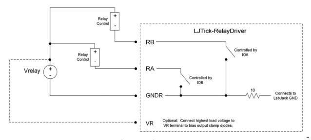
**Figure 5: General Connection Diagram**
