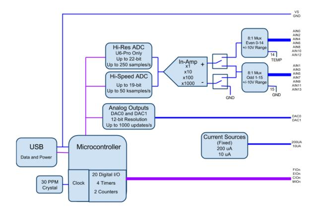
Figure 2-2. Block Diagram
