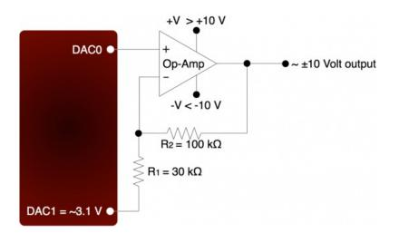
Figure 2.7.1.2-1. ±10 Volt DAC Output Circuit
