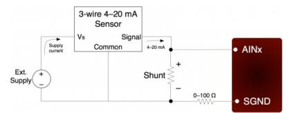
Figure 2.6.3.7-2. Current Measurement With 3-Wire 4-20 mA (Sourcing) Sensor
