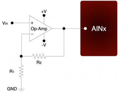
Figure 2.6.3.5-1. Non-Inverting Op-Amp Configuration
