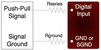
Figure 2.8.1.1-1. Driven Signal Connection To Digital Input
