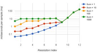
Figure B-2. Analog input effective resolution over various gains and resolution index settings.
