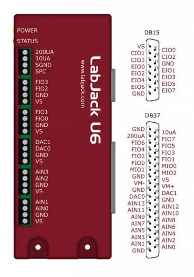
Figure 2-1. Enclosure & Connectors
