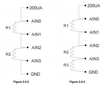
Figure 2.5-3 shows a setup to measure 2 resistors using differential analog inputs. AIN3 is wasted in this case, as it is connected to ground, so a differential measurement of AIN2-AIN3 is the same as a single-ended measurement of AIN2. That leads to Figure 2.5-4, which shows R1 and R2 measured differentially and R3 measured single-ended.
