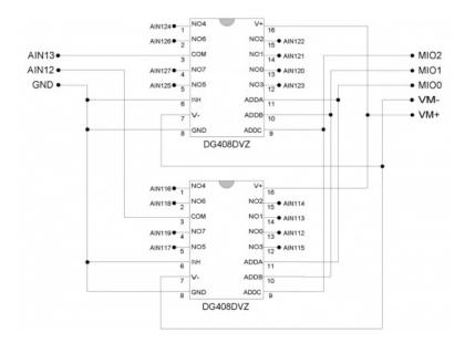
Figure 2-2. Typical External Multiplexer Connections
