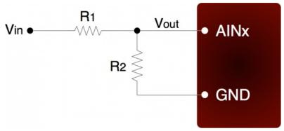
Figure 2.6.3.6-1. Voltage Divider Circuit
