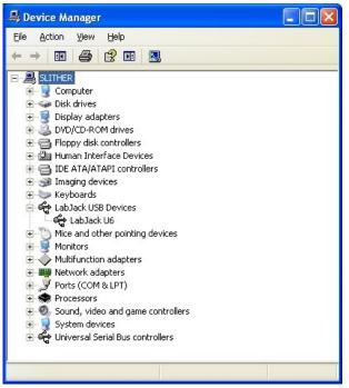
Correctly Functioning U6 in Windows Device Manager
