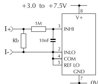
Measuring a current from a circuit which is floating with respect to the DPM's supply, i.e. the current and the meter's power supply are isolated from each other.
