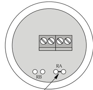
Cut the PCB track across Ra before fitting Ra.
