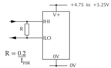
Measuring current. The meter's supply is isolated from the current being measured. Ensure Jumper link J1 is fitted. Ensure Jumper link J2 is not fitted.
