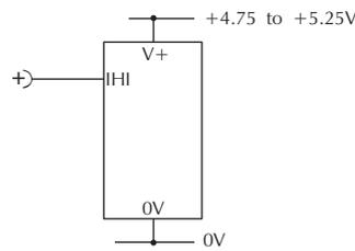
Measuring a single ended input voltage referenced to supply, i.e. the input voltage and the meter's power supply share the same 0V rail. Ensure Jumper link J1 is not fitted. Ensure Jumper link J2 is fitted.
