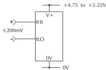
Measuring an input voltage referenced to a floating supply, i.e. the input voltage and the meter's power supply are isolated from each other. Ensure Jumper link J1 is fitted. Ensure Jumper link J2 is not fitted.
