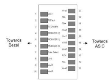
Pin-out of connector Block on Host board
