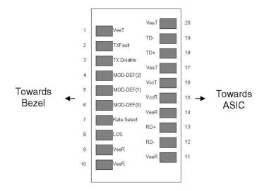
Pin-out of connector Block on Host board
