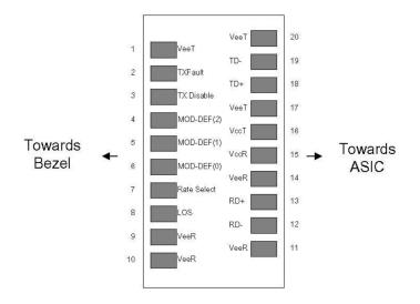
Pin-out of connector Block on Host board
