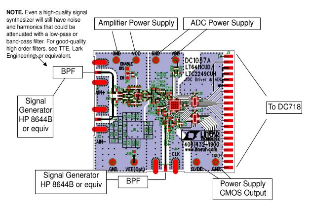
Figure 1. Proper Evaluation Equipment Setup
