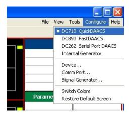
Figure 5. Selecting the correct input to QuickEval-II
