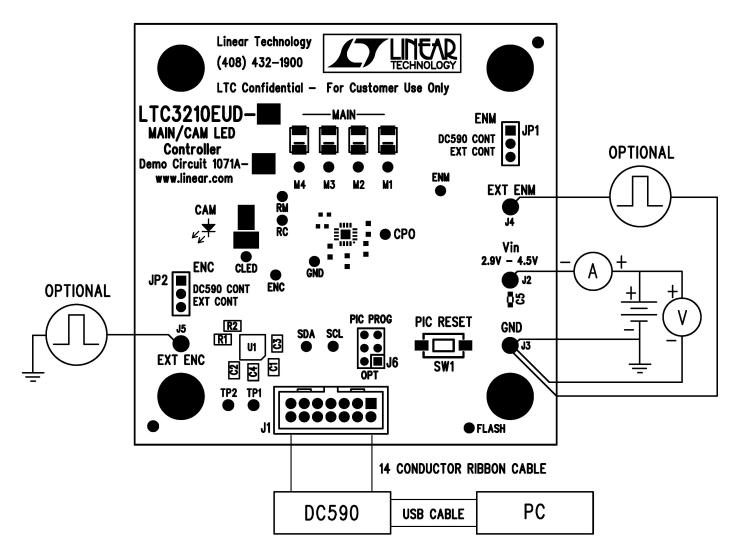
Figure 1. Proper Measurement Equipment Setup for DC1071A
