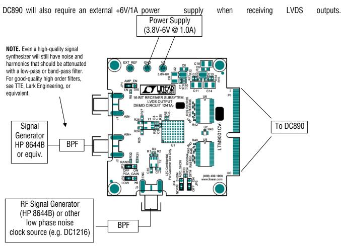
Figure 1. Proper Evaluation Equipment Setup
