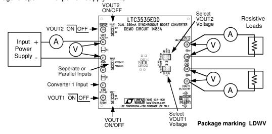
Figure 1. Demonstration Circuit Test Setup
