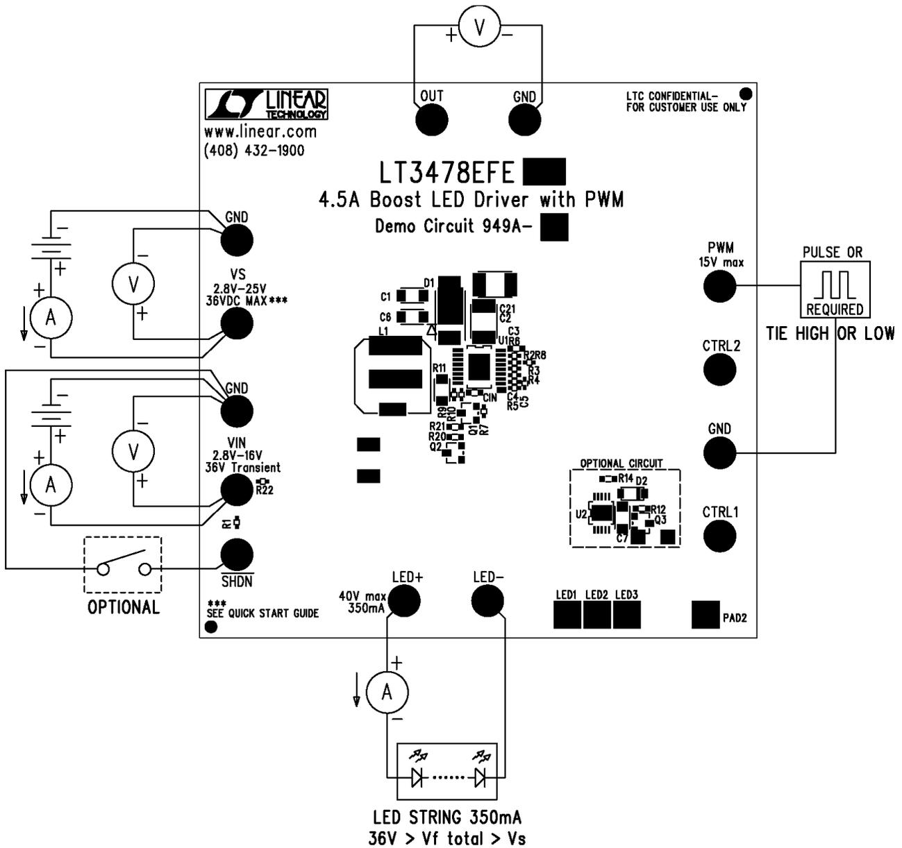
Figure 1. Test procedure setup drawing for DC949A-A DC949A-B
