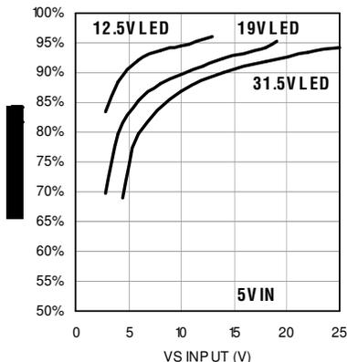
Figure 2. DC949A-A efficiency
