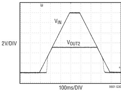
**Channel 2 Start-Up and Dropout,  $R_L = 20\Omega$**
