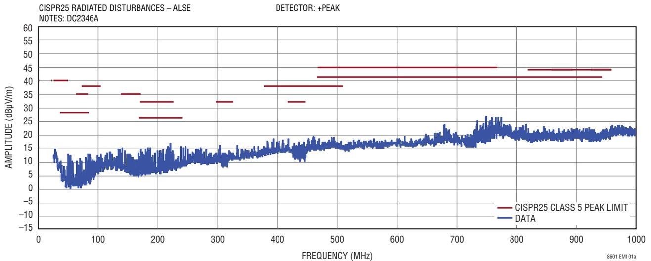
Demo Board with EMI Filter Installed,  $14V_{IN}$ , 1A on All Outputs,  $f_{SW} = 2\text{MHz}$ .
