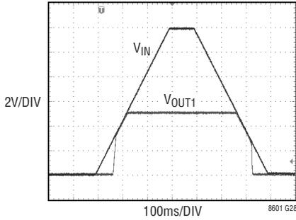
**Channel 1 Start-Up and Dropout,  $R_L = 3.3\Omega$**
