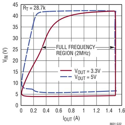
**Channel 2 Full Frequency  $V_{IN}$  vs Load Current**
