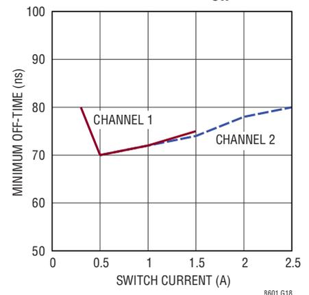
**TYPICAL PERFORMANCE CHARACTERISTICS**  $T_A = 25^\circ\text{C}$ ,  $V_{IN} = PV_{IN1} = PV_{IN2} = 12\text{V}$ ,  $EN/UVLO = 3\text{V}$  and  $PV_{IN3} = 3.3\text{V}$ , unless otherwise noted.
