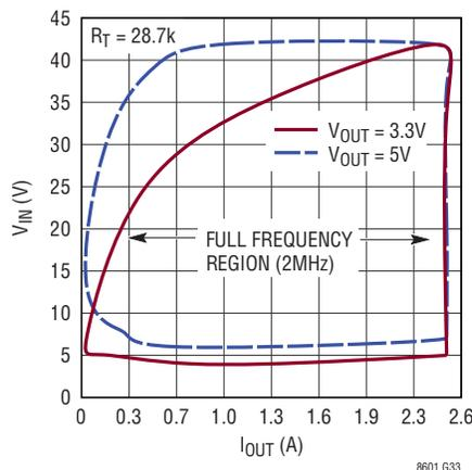
**Channel 3 Full Frequency  $V_{IN}$  vs Load Current**
