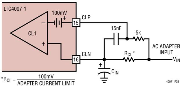
Figure 8. Adapter Current Limiting
