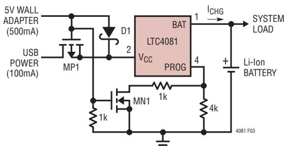
Figure 3. Combining Wall Adapter and USB Power
