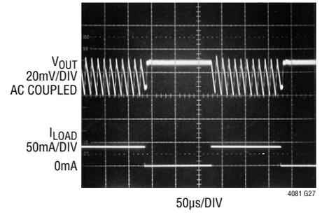
**Buck  $V_{OUT}$  Soft-Start ( $I_{LOAD} = 50\text{mA}$ )**
