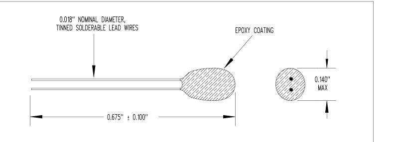
RESISTANCE @  $+25^{\circ}$ C = 10,000  $\Omega$  ± 1% RESISTANCE/TEMPERATURE CURVE = "J" BETA " $\beta$ " (0 TO  $+50^{\circ}$ C) = 3,892'K NOMINAL TEMPERATURE COEFFICIENT @  $+25^{\circ}$ C = -4.4%/'C NOMINAL DISSIPATION CONSTANT = 2 mW/'C NOMINAL THERMAL TIME CONSTANT = 15 SECONDS NOMINAL (STILL AIR) THERMAL TIME CONSTANT = 3 SECONDS MAXIMUM (STIRRED OIL) MAXIMUM TEMPERATURE RATING =  $+125^{\circ}$ C
