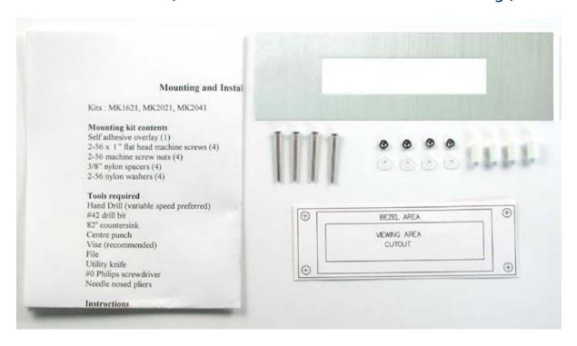
Mount a 20 character x 2 line display (Product # LK/ VK202-25 or LK/ VK/202-25-USB or MOS/ MOI/ MOU-AL/ VK202A) just about anywhere with this kit. Place the self-adhesive overlay on the surface where you'd like to mount the display; use it as a guide for cutting out a window for the display and drilling holes for the mounting screws. Includes: Self-adhesive overlay, adhesive cut and drill guide.
