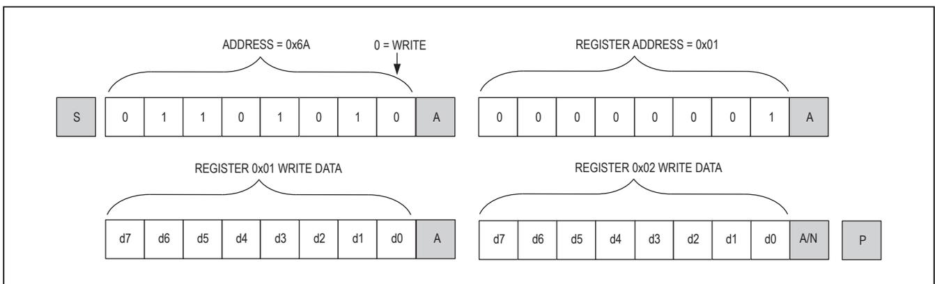
Figure 9. Format for Writing to Multiple Registers
