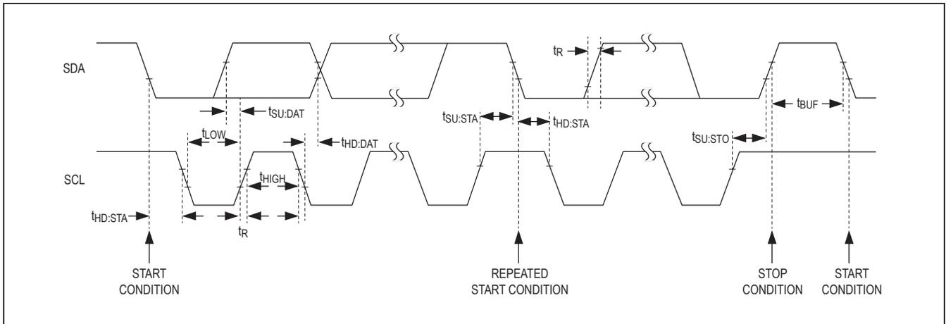
Figure 3. I<sup>2</sup>C Interface Timing
