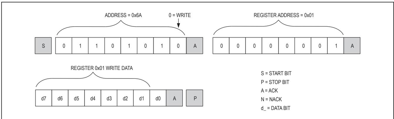
Figure 8. Format for I<sup>2</sup>C Write
