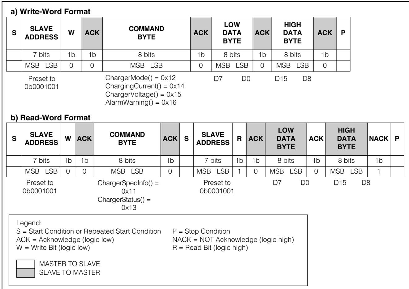
Figure 3. SMBus a) Write-Word and b) Read-Word Protocols
