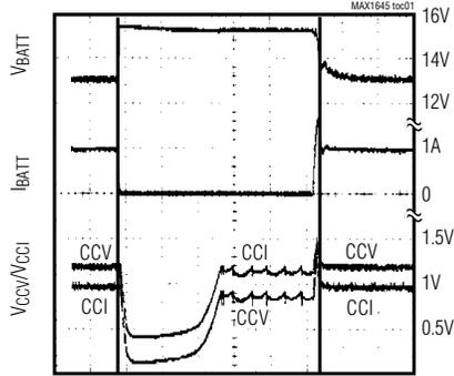
BATTERY REMOVED 2ms/div BATTERY INSERTED
