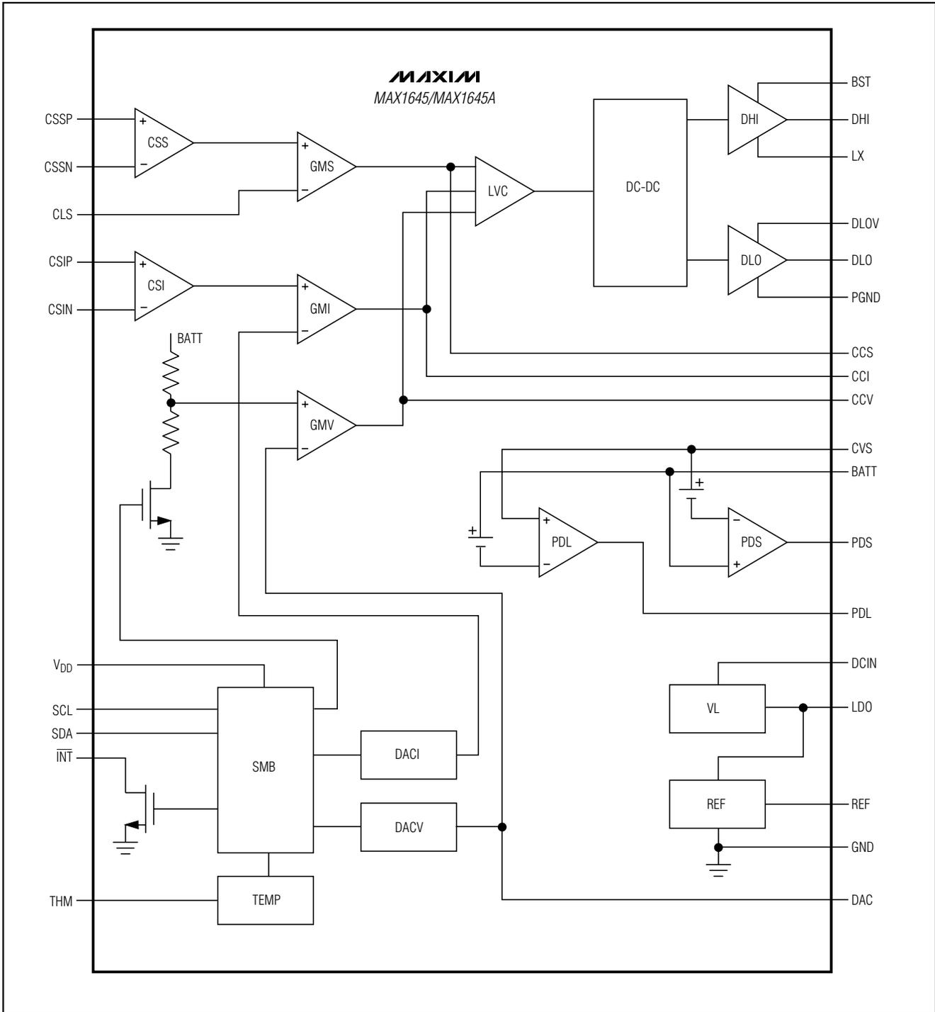
Figure 2. Functional Diagram
