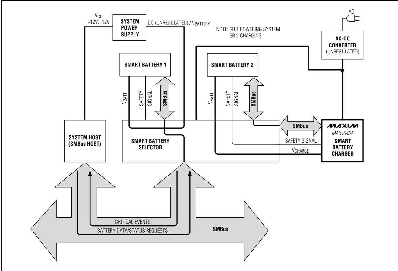
Figure 11. Typical System Using Multiple Smart Batteries
