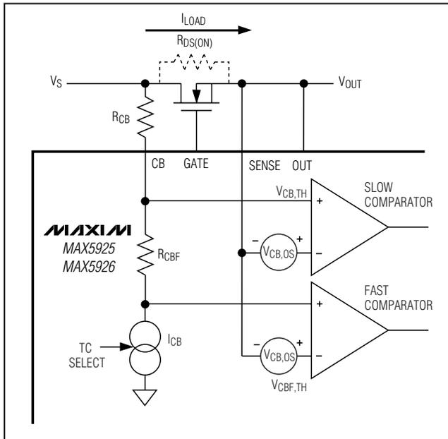
Figure 12. Circuit Breaker Using  $R_{DS(ON)}$
