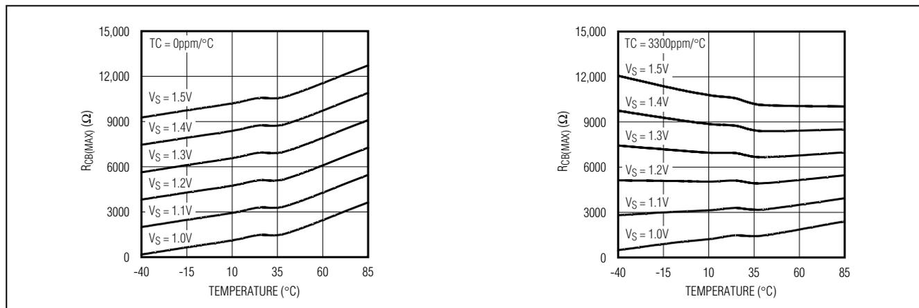
Figure 11. Maximum Circuit-Breaker Programming Resistor vs. Temperature
