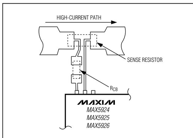
Figure 15. Kelvin Connection for the Current-Sense Resistor
