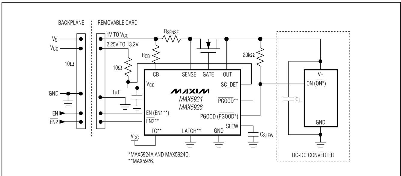
Figure 2. Typical Operating Circuit (With  $R_{SENSE}$ )
