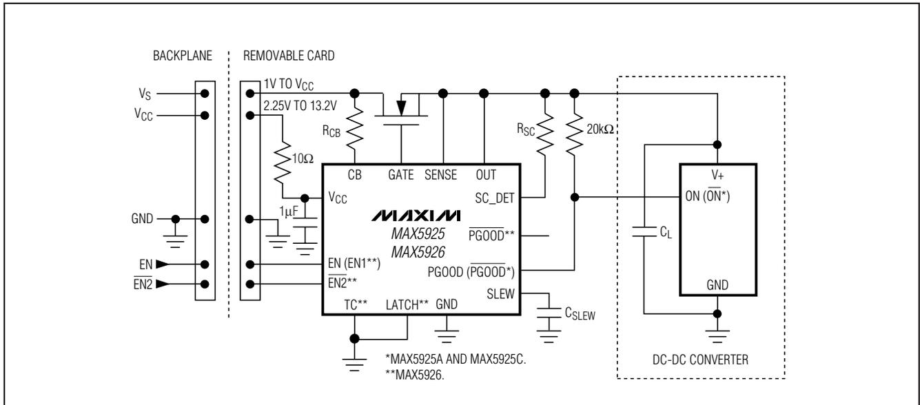
Figure 1. Typical Operating Circuit (Without  $R_{SENSE}$ )
