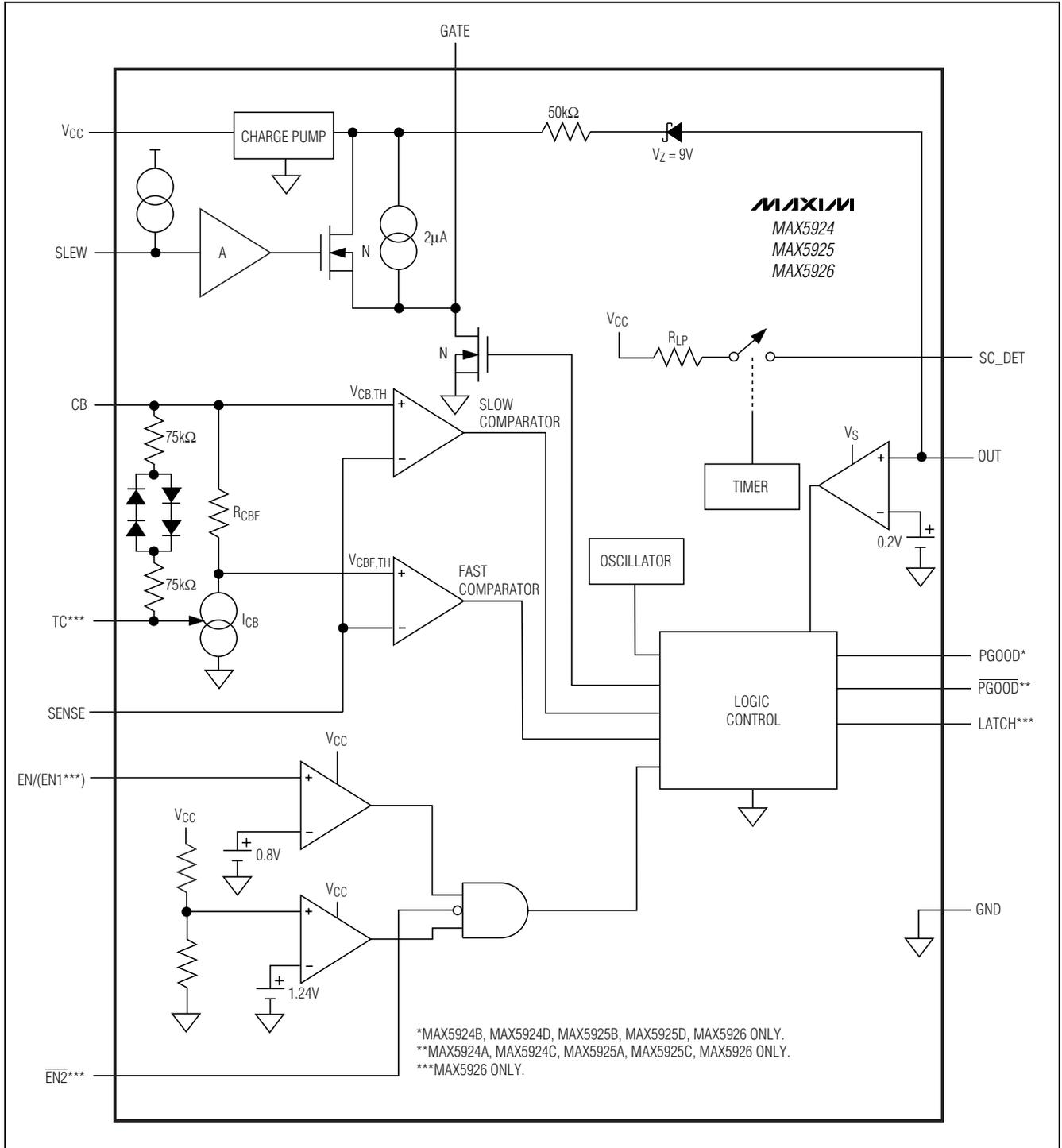
Figure 3. Functional Diagram
