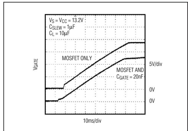
Figure 9. Impact of  $C_{GATE}$  on the  $V_{GATE}$  Waveform
