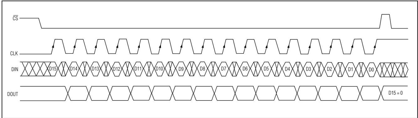
Figure 4. Transmission of 16 Bits to the MAX6954
