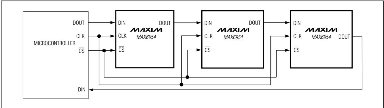
Figure 2. MAX6954 Daisy-Chain Connection
