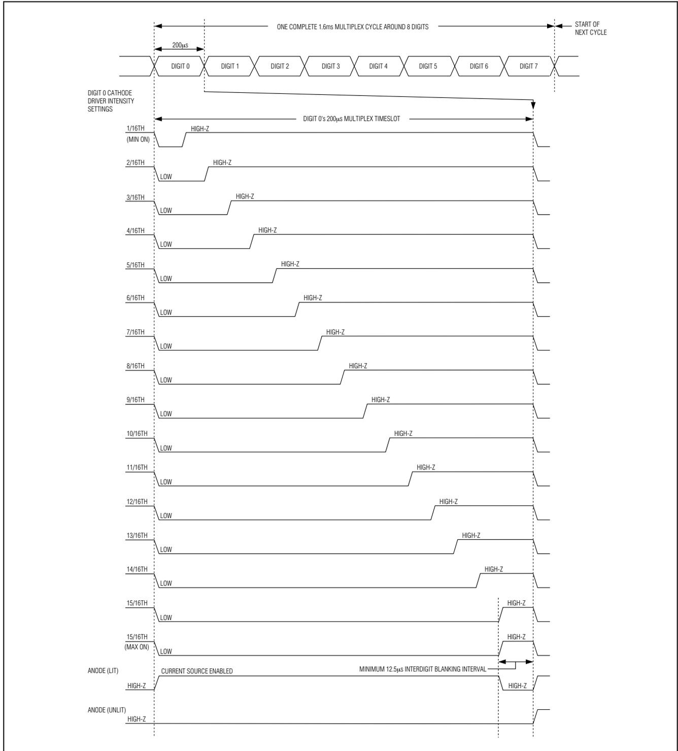
Figure 6. Multiplex Timing Diagram (OSC = 4MHz)
