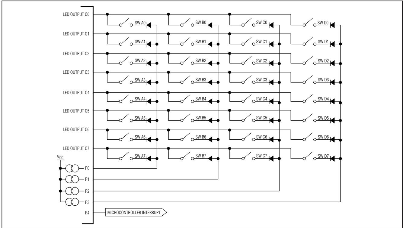
Figure 7. Key-Scanning Configuration
