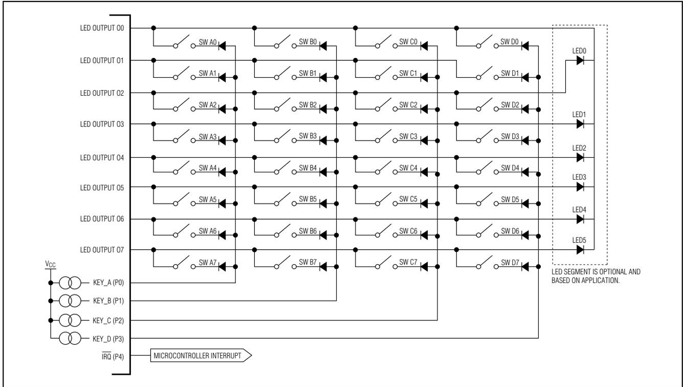
Figure 11. Key-Scanning Configuration
