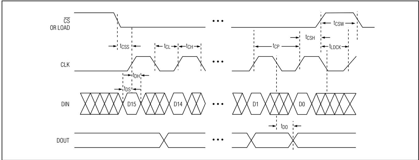
Figure 1. Timing Diagram
