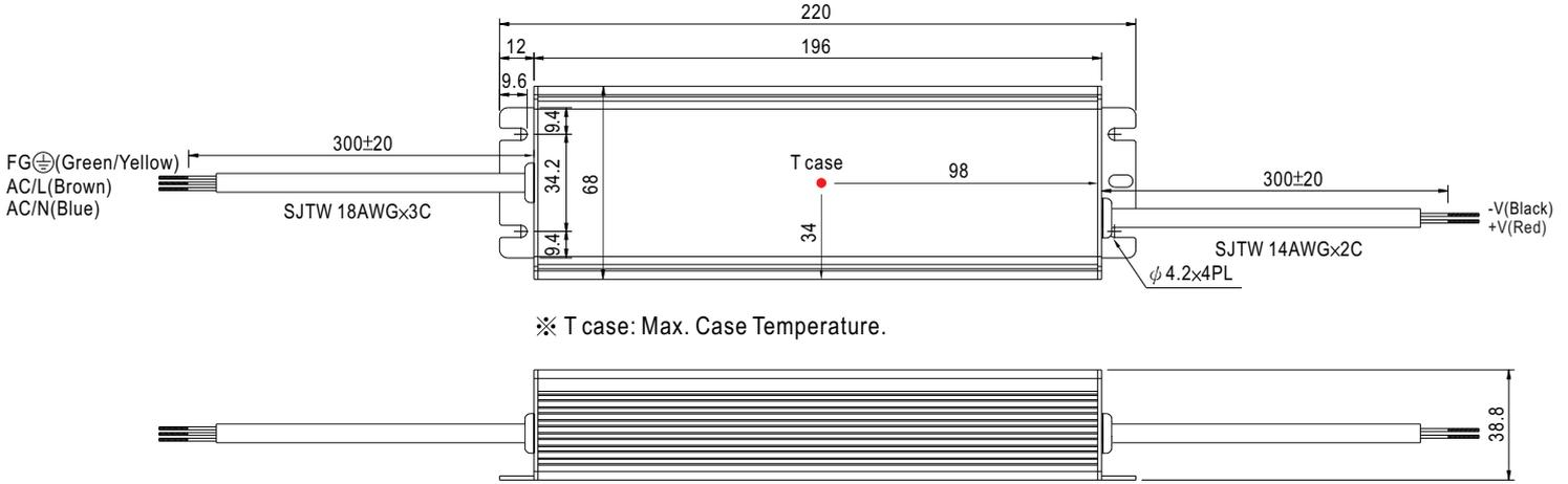
※ IP67 rated. Timer dimming function, contact MEAN WELL for details.
