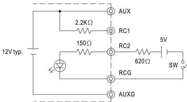
(B) Using internal 12V auxiliary output
