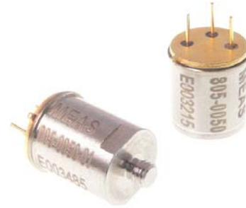
**The Model 805** is a miniature adhesive mount IEPE accelerometer built on a 3-pin TO-5 header. It is available in  $\pm 50g$  and  $\pm 500g$  dynamic ranges and offers a flat frequency response to 15kHz. The accelerometer features a hermetic construction in a TO-5 header configuration. The model 805 incorporates a stable piezo-ceramic crystal and an integrated charge converter amplifier in a 100% shielded housing suitable for many embedded OEM applications.
