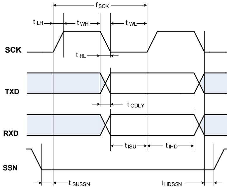
**Table 10-4. SPI Slave Timing Parameters<sup>1</sup>**
