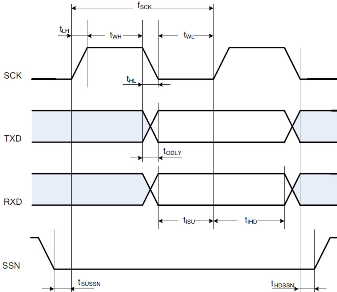
The following table provides the SPI Slave timing parameters for the ATWINC3400-MR210CA module.
