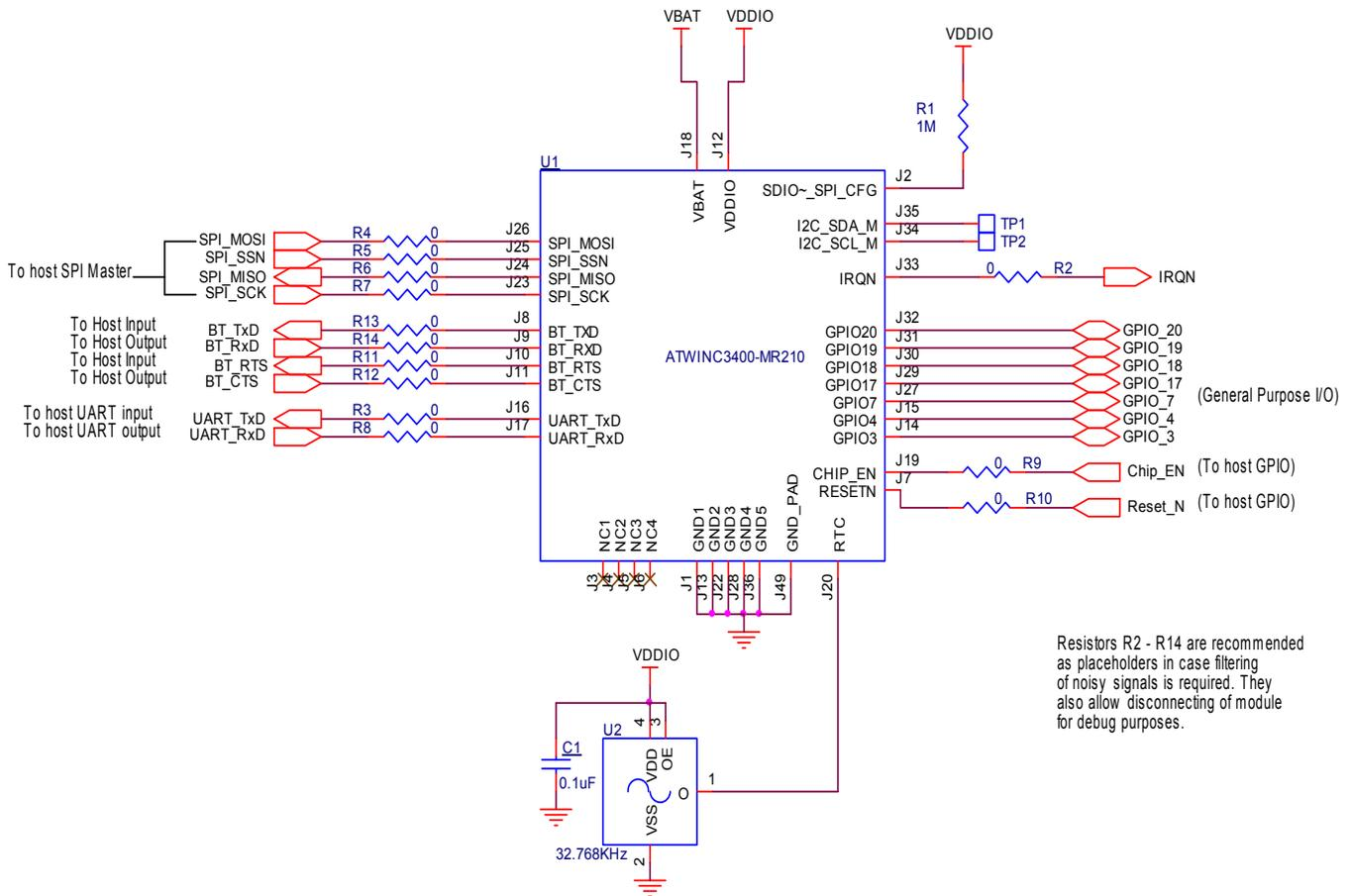
**Note:** It is recommended to add test points for module pins J8, J9, J10, J11, J16 and J17 in the design.
