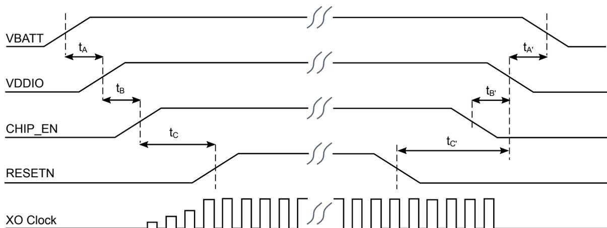
The following table provides power-up/down sequence timing parameters.
