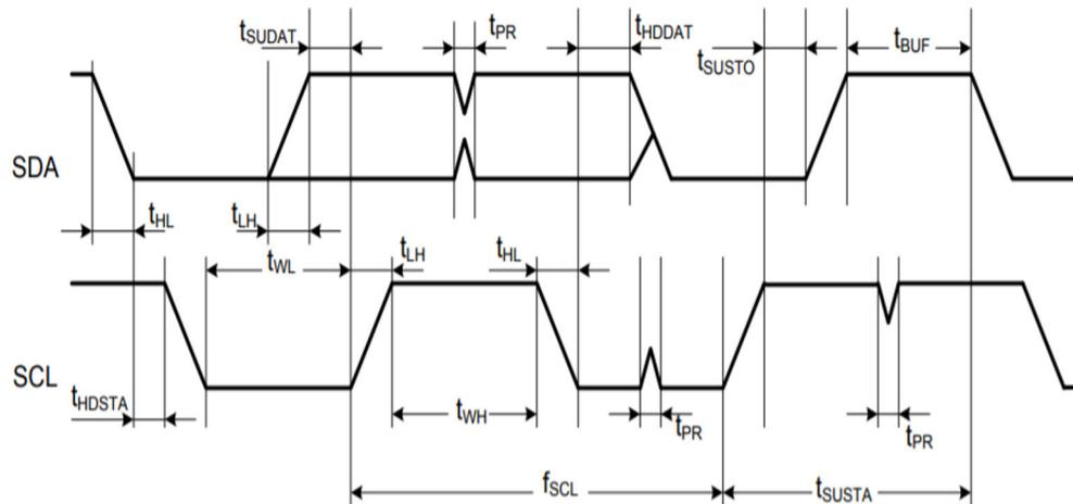
The following table provides the I<sup>2</sup>C Slave timing parameters for the ATWINC3400-MR210CA module.
