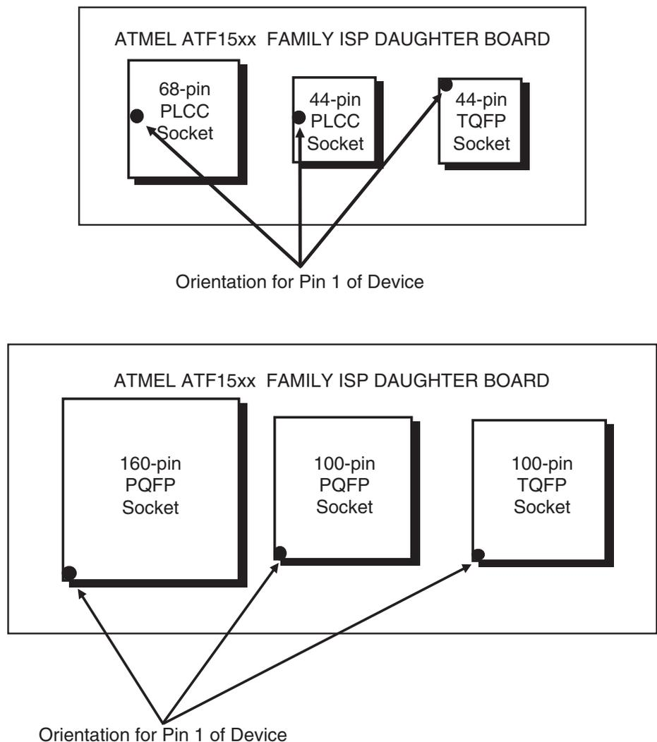
**Figure 4-4.** Correct Orientation of Daughter Board on ISP Board
