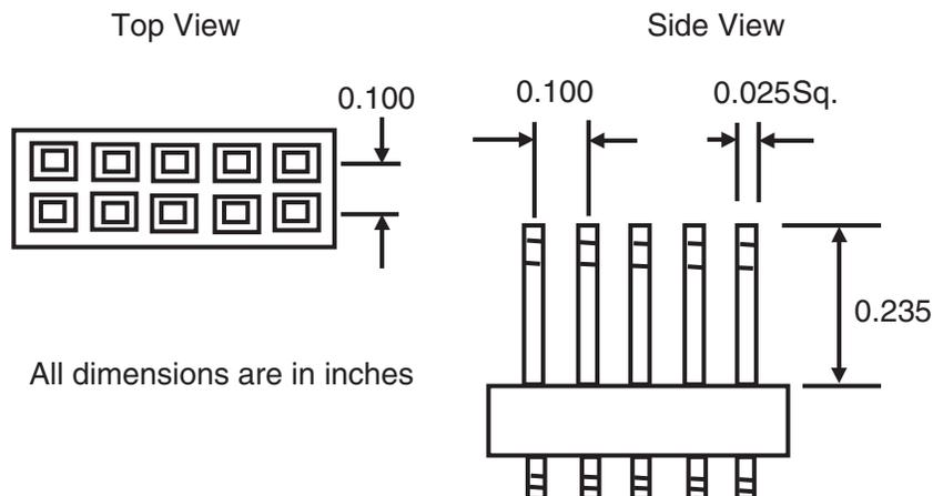
**Figure 4-8.** 10-pin Male Header Pinout
