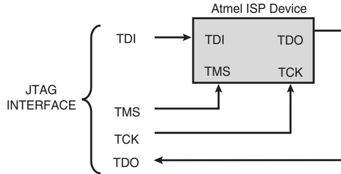
**Note:** You will need to reserve space on your circuit board to accommodate a 10-pin male header for the JTAG interface. The pinout for this header must match the Atmel-ISP cable connector pinout. The JTAG interface pins for each Atmel device must also be connected to this header.
