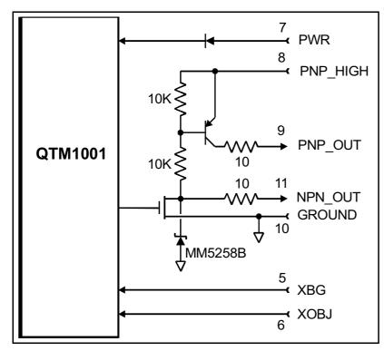
The QTM has simultaneous PNP and NPN outputs; the PNP high voltage (pin 8) is usually strapped to Power (pin 7), but in some cases, for example for logic level compatibility, it may be desirable to strap it to +5 or some other voltage.
