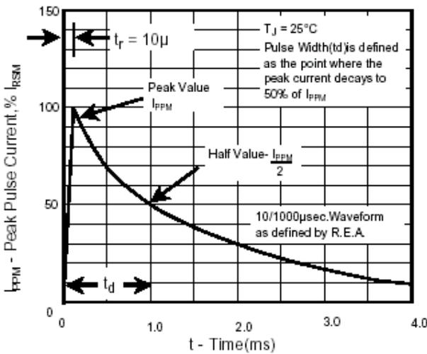
Fig.4 - Maximum Non-Repetitive Forward Surge Current Uni-Directional Only
