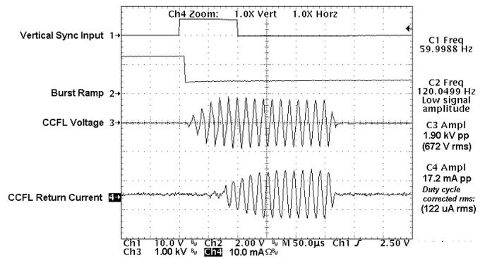
Figure 3 – 2% Burst Duty Cycle (Expanded Time Base)
