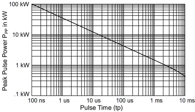
**FIG. 1 – Non-repetitive peak pulse power rating curve**
