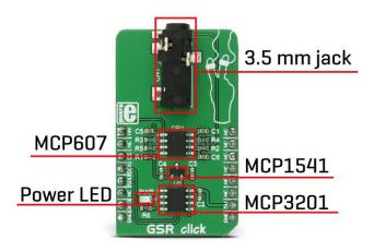
GSR click uses the MCP607, a dual CMOS low-noise OPAMP made by Microchip, as well as the MCP3201, a 12bit SAR type ADC, made by the same company. The input stage consists of the aforementioned voltage divider and a frequency limiting capacitor. This signal is then fed to the first half of the OPAMP, set to a unity gain. It is used to condition the signal before entering the ADC.
