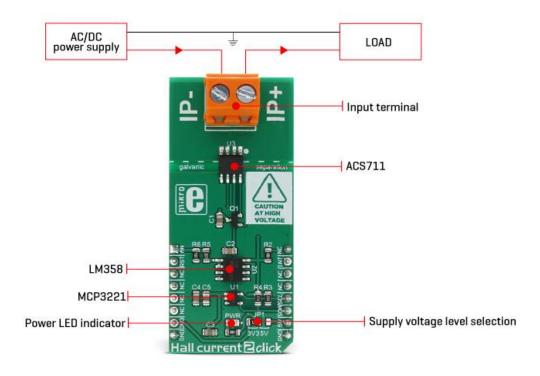
The output voltage changes linearly with the input current, in steps of 110mV/A. To allow conversion via the external ADC, the output voltage is passed through the buffering circuit, comprised of the LM358 - a low noise operational amplifier in a unity gain configuration.
