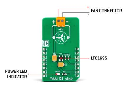
Brushless motors can sometimes exhibit the stall effect if started with the reduced voltage. Although the fan will not rotate, the current will still be consumed, making the stall condition sensing difficult. Therefore, the
