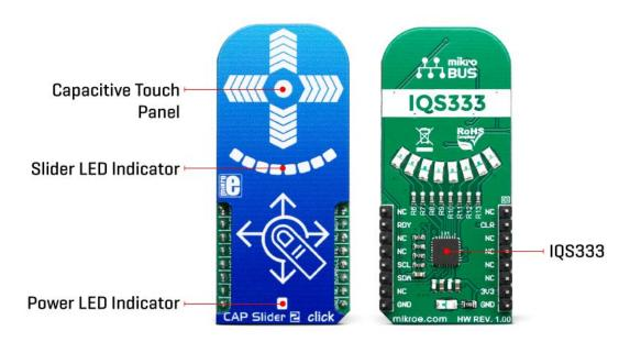
Capacitive touch sensing is based on detecting a change in capacitance, due to the influence of a foreign object. Basically, the capacitance of the sensor, also known as the
