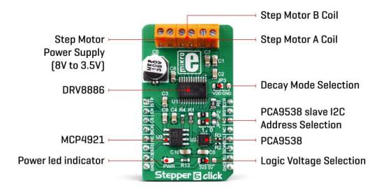
The high efficiency of the integrated N-Channel power MOSFET H-Bridges allows a high efficiency to be achieved: Stepper 6 click can withstand peaks of current up to 3A, while the internal current limiter is set to 1.4 A per
