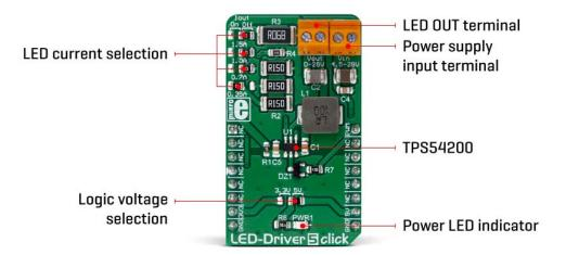
The PWM pin is used to control more than just one function. Besides choosing the dimming mode (analog or PWM), this pin is also used to enable or disable the IC. If the signal at the PWM pin rises above the threshold value (0.56V typically) the IC will be enabled. Keeping the voltage at the PWM pin lower than 0.56V for at least 40 ms will effectively disable the IC.
